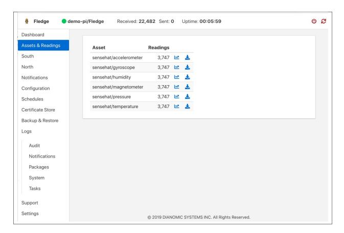
You can inspect all the data buffered by the Fledge system on the Assets page. To access this page, click on "Assets & Readings" from the left-side menu bar.
