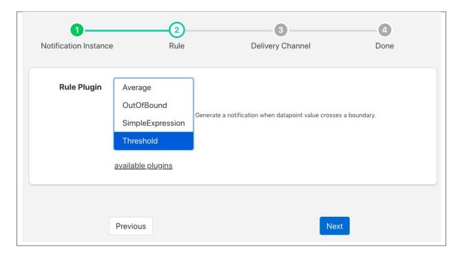
You are presented with the set of installed rules on the system. If the rule you wish to use is not installed and you wish to install it then use the link *available plugins* to be presented with the list of plugins that are available to be installed.
