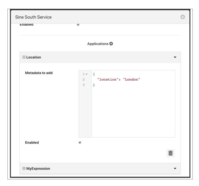
You can also remove a filter from the pipeline of filters by select the trash can icon at the bottom right of the edit area for the filter.
