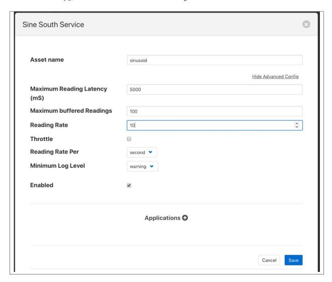
Amongst the advanced setting you will see one labeled *Reading Rate*. This defaults to 1 per second. The sinusoid takes 60 samples to complete one cycle of the sine wave, therefore it has a periodicity of 1 minute, or 0.0166Hz. If the *Reading Rate* is st to 60, then the frequency of the output becomes 1Hz.
