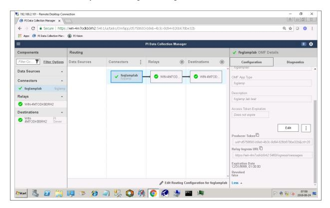
Finally, select the new Fledge application. Click "More" at the bottom of the Configuration panel. Make note of the Producer Token and Relay Ingress URL.
