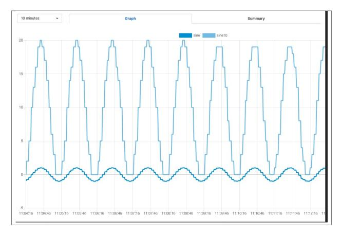
Some jitter caused by occasional differences in the readings that arrive in a single block can be seen in the data as well.
