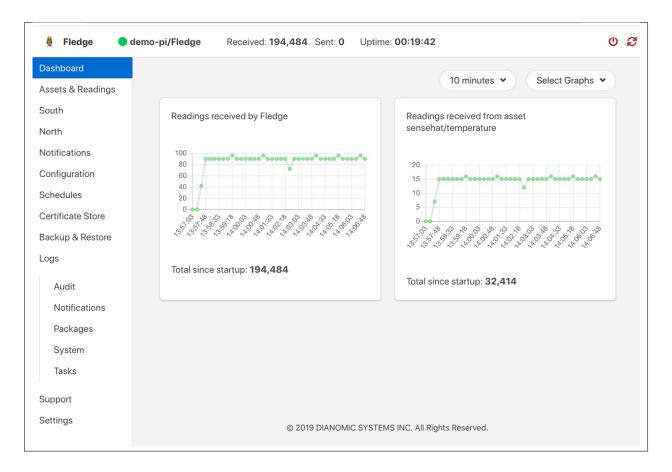
This screen provides an overview of Fledge operations. You can customize the information and time frames displayed on this screen using the drop-down menus in the upper right corner. The information you select will be displayed in a series of graphs.
