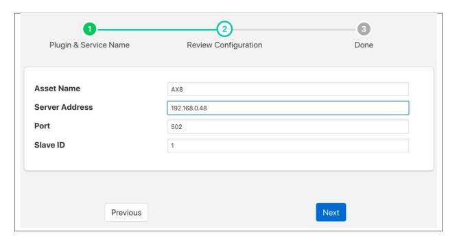
There are four configuration parameters that can be set, usually it is only necessary to change the first two however;
