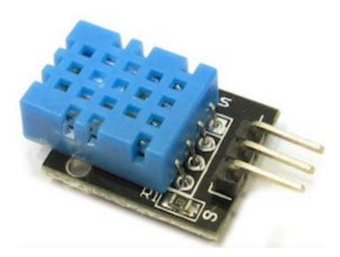
The *fledge-south-dht* plugin implements a temperature and humidity sensor using the DHT11 sensor module. Two versions of plugins for the DHT11 are available and are used as the example for . The other DHT11 plugin is *fledge-south-dht11* and is a .
