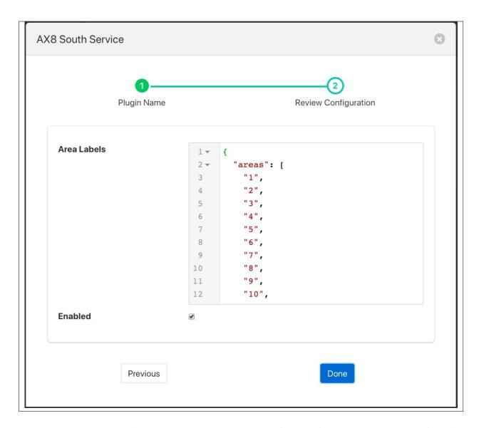
The JSON document *Area Labels* can be used to set the labels to use for each of the boxes and replace the min1, min2 etc. The value of this configuration option is a JSON document that has a single element called *areas* which is a JSON array. Each element in that area is the name to assign to the particular box. The default values would set the name of box1 to simply be 1, box2 to 2 etc.
