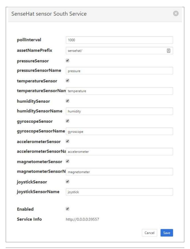
To modify the configuration of a data source, click on its name in the South Services screen. This will display a list of all parameters available for that data source. If you make any changes, click on the "save" button in the top panel to save the new configuration. Click on the "x" button in the upper right corner to return to the South Services screen.
