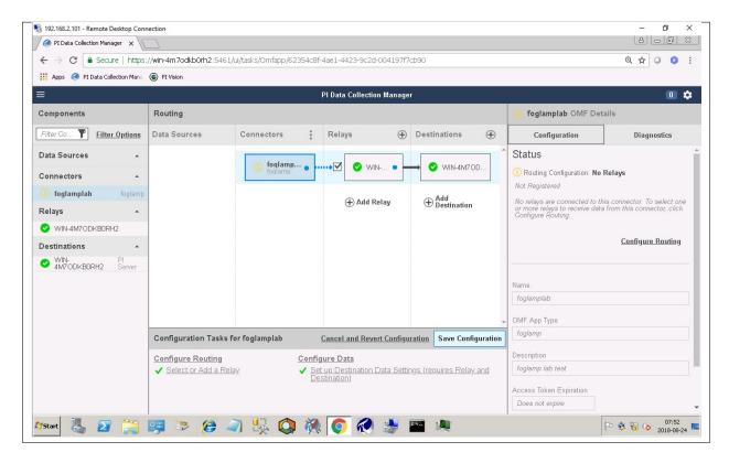
Connect the new application to the PI Connector Relay by selecting the new Fledge application, clicking the check box for the PI Connector Relay and then clicking "Save Configuration".
