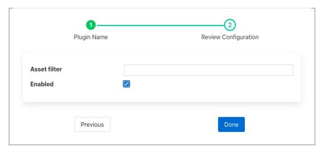
The Asset Filter entry is a regular expression that can be used to limit the assets that the filter will effect. To change all assets leave this entry blank.
