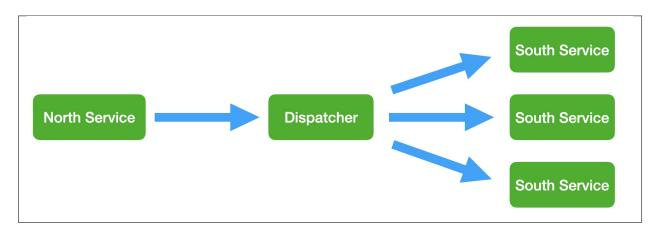
It is the job of the north plugin to define how the control input is received, as this is specific to the protocol of device to the north of Fledge. The plugin then takes this input and maps it to a control message that can be routed by the dispatcher. The way this mappings is defined is specific to each of the north plugins that provide control input.
