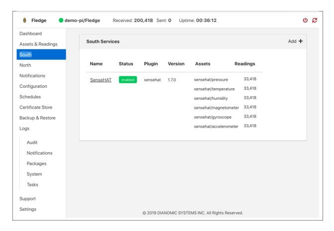
Data sources are managed from the South Services screen. To access this screen, click on "South" from the menu bar on the left side of any screen.
