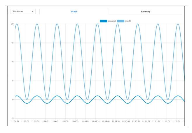
The data observed that is written to the modbus device is not however a clean sine wave as readings have been missed due to the retrigger time eliminating data that arrived in the same buffer.
