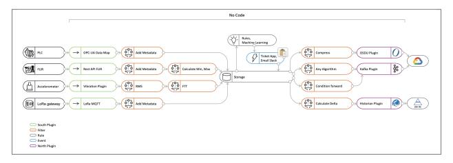
This allows for data processing to be built up via the graphical interface of Fledge with little or no coding required. Filters that are applied in a south service will affect all out going streams whilst those applied in the north only affect the data that is sent on that particular connection to an external system.
