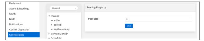
• **Pool Size**: The storage service uses a connection pool to communicate with the underlying database, it is this pool size that determines how many parallel operations can be invoked on the database.
