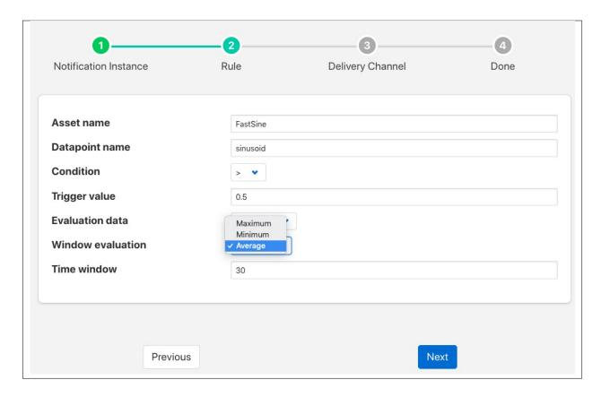
Once you have set the parameters for the rule click on the *Next* button to select the delivery plugin to use to delivery the notification data.
