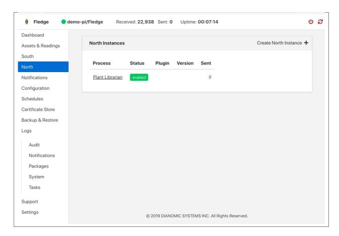
Data destinations are managed from the North Services screen. To access this screen, click on "North" from the menu bar on the left side of any screen.
