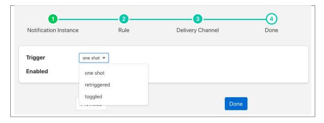
The final stage of setting up your configuration is to set the notification type and the retrigger time for the notification. Enable the notification and click on *Done* to complete setting up your notification.
