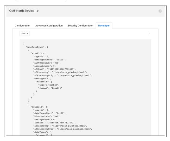
It is possible for more than one plugin within a pipeline to persist data, in order to select between the plugins that have persisted data a menu is provided in the top left which will list all those plugins for which data can be viewed.
