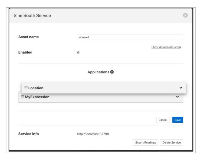
Filters are executed in a top to bottom order always. It may not matter in some cases what order a filter is executed in, in others it can have significant effect on the result.
