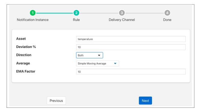
The Asset entry field is used to define the single asset that the plugin should monitor.
