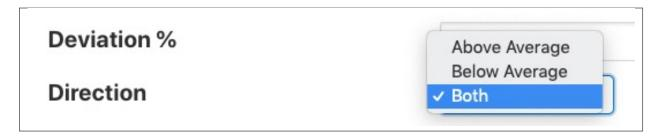
The *Direction* entry is used to define if the rule should trigger when the current value is above average, below average or in both cases.
