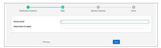
The *Asset* entry field is used to define the single asset that the plugin should monitor.
