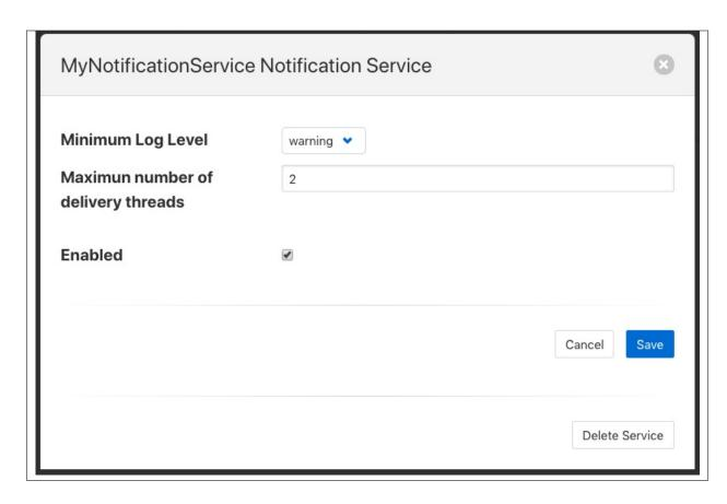
You can use this dialog to control the level of logging that is done from the service by setting the *Minimum Log Level* to the least severity log level you wish to see. All log entries at the select level and of greater severity will be logged.
