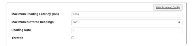
The above shows the default configuration of a south service. In this case data will not be sent to the south service until there are either 100 readings buffered in the south service, or the oldest reading in the south service buffer has been in the buffer for 5000 milliseconds. In this example we are reading 1 new readings every second, therefore will send data to the storage service every 5 seconds, when the oldest reading in the buffer has been there for 5000mS.
