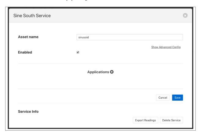
Towards the bottom of this dialog is a section labeled *Applications* with a + icon to the right, select the + icon to add a filter to the south service. A filter wizard is now shown that allows you to select the filter you wish to add and give that filter a name.
