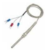
The *fledge-south-pt100* is a south plugin for the PT-100 temperature sensor. The PT100 is a resistance temperature detectors (RTDs) consist of a fine wire (typically platinum) wrapped around a ceramic core, exhibiting a linear increase in resistance as temperature rises. The sensor connects via a MAX31865 converter to a GPIO pins for I2C bus and a chip select pin.
