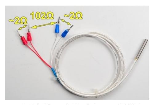
To connect a three wire sensor connect the red pair of wires across the RTD+ pair of connectors and the third wire on the RTD- block. If your PT100 doe not have a pair of red wires, or you wish to verify the colours and have access to a multimeter, the resistance between the red wires should be 2 ohms. ~The resistance to the third wire, from the red pair, will be approximately 102 ohms but will vary with temperature.
