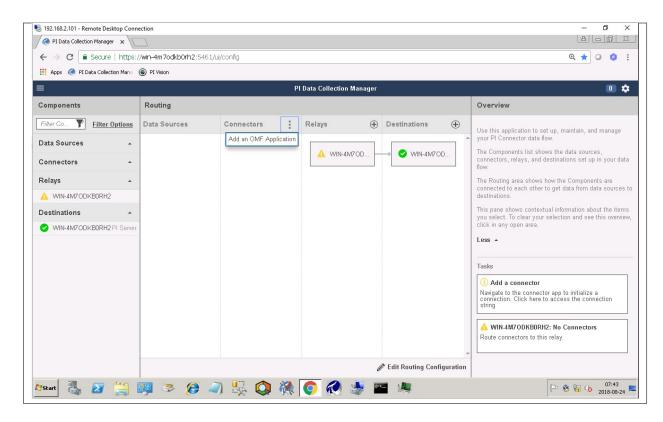
To add a new connector for the Fledge system, click on the drop down menu to the right of "Connectors" and select "Add an OMF application". Add and save the requested configuration information.
