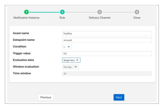
You will be presented with the configuration parameters applicable to the rule you have chosen. Enter the name of the asset and the datapoint within that asset that you wish the rule to operate on. In the case of the *threshold rule* you can also define if you want the rule to trigger if the value is greater than, greater than or equal, less than or less than or equal to a *Trigger value*.
