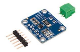
The *fledge-south-ina219* plugin is a south plugin that uses an INA219 breakout board to measure current and voltage. The Texas Instruments INA219 is capable of measuring voltages up to 26 volts and currents up to 3.2 Amps. It connects via the I2C bus of the host and multiple sensors may be daisy chain on a single I2C bus. Breakout boards that mount the chip and its associate shunt resistor and connectors and easily available and attached to hosts with I2C buses.
