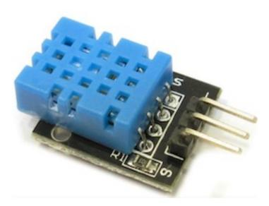
The *fledge-south-dht* plugin implements a temperature and humidity sensor using the DHT11 sensor module. Two versions of plugins for the DHT11 are available and are used as the example for . The other DHT11 plugin is *fledge-south-dht11* and is a .
