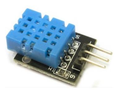
The fledge-south-dht11 plugin implements a temperature and humidity sensor using the DHT11 sensor module. Two versions of plugins for the DHT11 are available and are used as the example for . The other DHT11 plugin is fledge-south-dht and is a .
