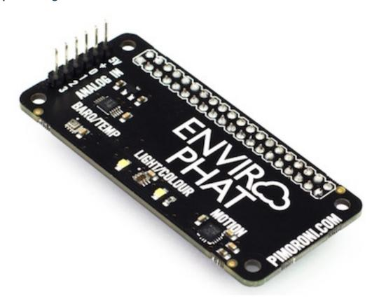
The *fledge-south-rpienviro* is a plugin that uses the Pimoroni Enviro pHAT sensor board. The Enviro pHAT board is an environmental sensing board populated with multiple sensors, the plugin pulls data from the;
