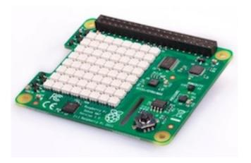
The *fledge-south-sensehat* is a plugin that uses the Raspberry Pi Sense HAT sensor board. The Sense HAT has an 8×8 RGB LED matrix, a five-button joystick and includes the following sensors:
