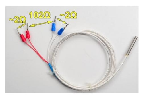
To connect a three wire sensor connect the red pair of wires across the RTD+ pair of connectors and the third wire on the RTD- block. If your PT100 doe not have a pair of red wires, or you wish to verify the colours and have access to a multimeter, the resistance between the red wires should be 2 ohms. ~The resistance to the third wire, from the red pair, will be approximately 102 ohms but will vary with temperature.
