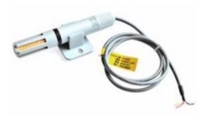
The *fledge-south-am2315* is a south plugin for a temperature and humidity sensor. The sensor connects via the I2C bus and can provide temperature data in the range  $-40^{\circ}$ C to  $+125^{\circ}$ C with an accuracy of  $0.1^{\circ}$ C.
