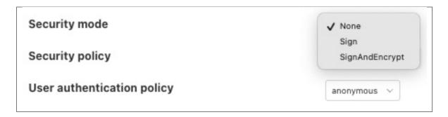
• Security Mode: Specify the OPC/UA security mode that will be used to communicate with the OPC/UA server.
