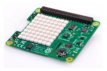
The *fledge-south-sensehat* is a plugin that uses the Raspberry Pi Sense HAT sensor board. The Sense HAT has an 8×8 RGB LED matrix, a five-button joystick and includes the following sensors:
