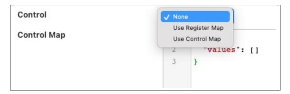
If no control is required then this may be set to *None*. Setting this to *Use Register Map* will cause all the registers that are being rad to also be targets for control. Setting this to *Use Control Map* will case the serperate *Control Map* to be used to map the control set points to modbus registers.
