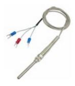
The *fledge-south-pt100* is a south plugin for the PT-100 temperature sensor. The PT100 is a resistance temperature detectors (RTDs) consist of a fine wire (typically platinum) wrapped around a ceramic core, exhibiting a linear increase in resistance as temperature rises. The sensor connects via a MAX31865 converter to a GPIO pins for I2C bus and a chip select pin.
